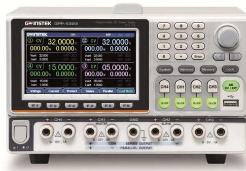
high program resolution (1mV/0.1mA) and read back resolution (0.1mV/0.1mA), but also features optimal low-ripple noise characteristics  $\leq 350\mu\text{Vrms}/\leq 2\text{mArms}$  and output transient recovery capability  $\leq 50\mu\text{s}$ . Independent output on-off switch is provided for each channel.
