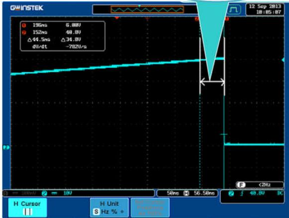
The protection mechanism of OVP/OCP/OTP is implemented by hardware circuit, which has the advantage of faster response time than competitors who use software to achieve protection. When it is detected that the voltage of the DUT exceeds the setting value of the OVP, the output of the power supply can be stopped in a short time to achieve the purpose of protecting the DUT.
